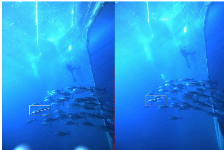
Figure 17. Example of incorrect measurement by the automatic software during first transfers in the Adriatic, where the snout point is placed on one fish and the fork point on a nearby fish.
