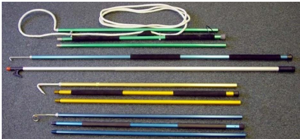
Figure 19 Long handled device (from top): turtle tether, J-Style de-hooker, line cutter and de-hooker for ingested hooks (Source NOAA).
