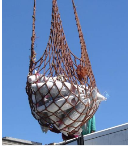
Figure 5 Fish being offloaded using a cargo net
