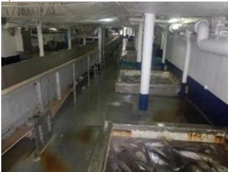
Figure 8 Fish hold and wells on a purse seine vessel (A) and hatch plan (B)
