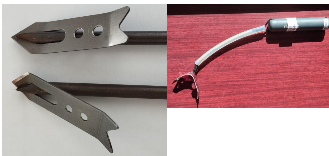
Figure 4 – Details on the Wildlife titanium anchor (top left) and stainless-steel anchor (bottom left) with Wildlife titanium applicator needle. The stainless-steel anchor (on the left) was correctly inserted but could not hold a traction force of approximately 40kg (right).
