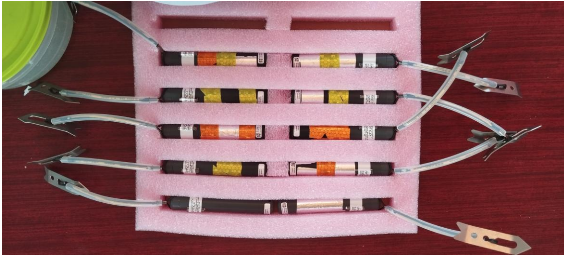
Figure 3 - Color combination using reflective tape to create uniquely identifiable patterns
