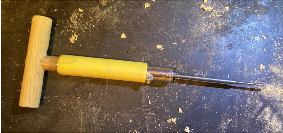
Figure 4. Tagging pole designed to insert the anchors with the fish inside the water
