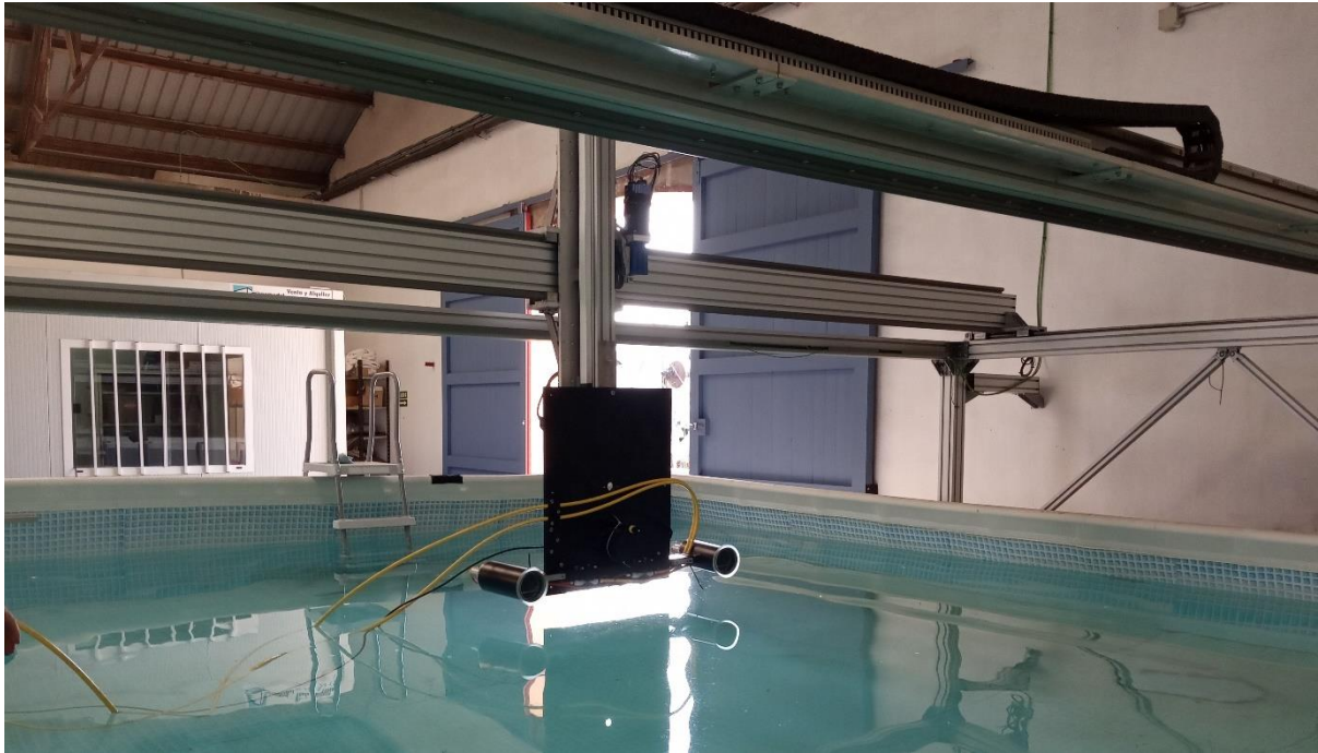
Figure 6. Picture taken during the calibration of the acoustic-optic relative transformation.
