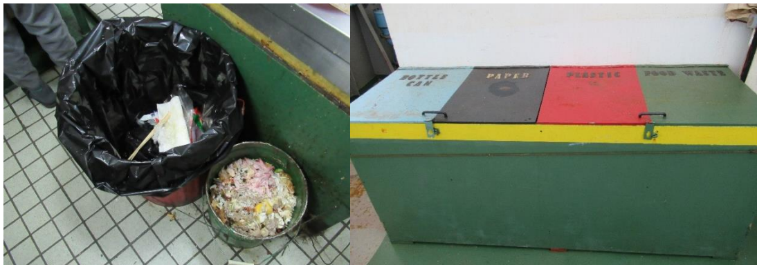
Figure 3 Galley waste and plastic & paper waste container situated in galley (left) and demarcated waste containers situated on aft deck.
