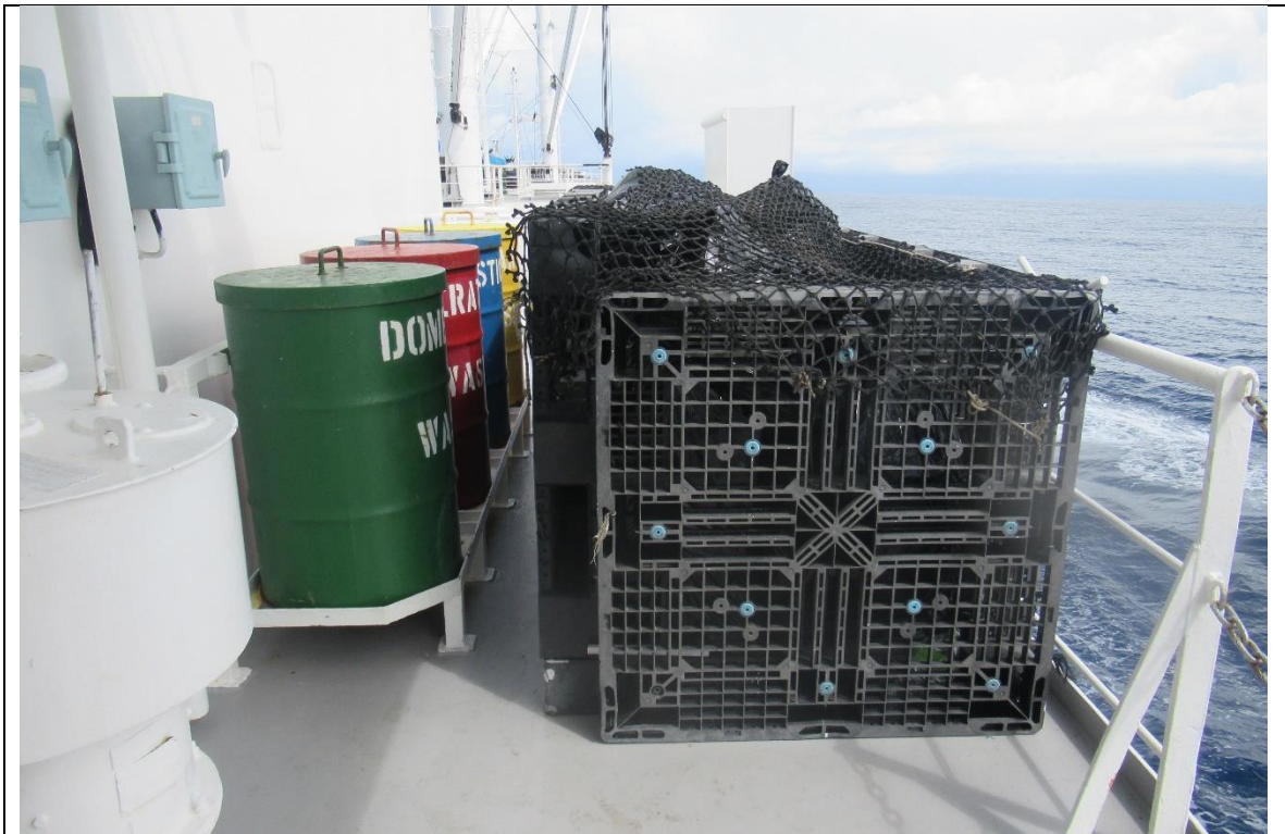
Figure 5: Garbage collection and separation system.
