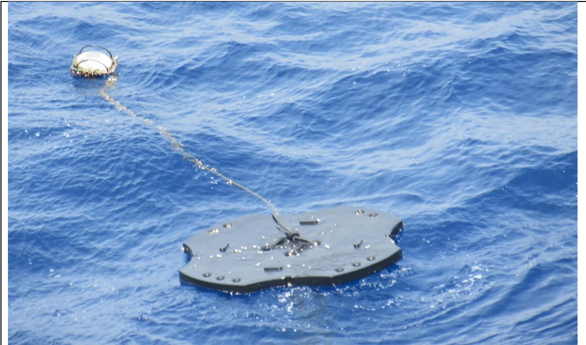
Figure 6: A FAD, NA1003BUOY, with GPS tracking device.
