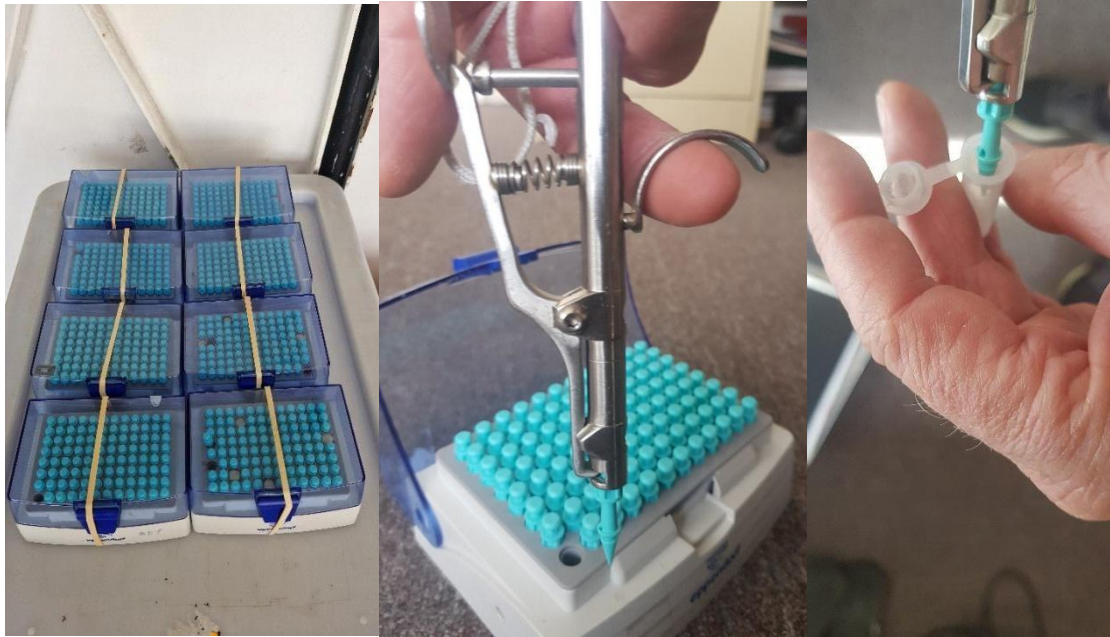
Figure 1. Left: tips loaded into boxes. Centre: Tip picked up by handle. Right: Tip with tissue dispensed into vial. Pictures from Russell Bradford – CSIRO
