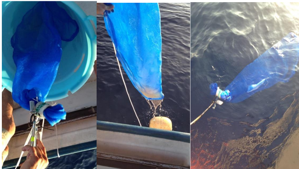
Figure 5. Alternative floating net in situ egg incubator. Eggs are deposited in the weighted net and hung vertically in the water. They were incubated for just over 24hrs and then reassembled for laboratory control and released. A plastic supporting frame has since been added recently to prevent net rubbing and a Hobo data logger was used to record temperature.
