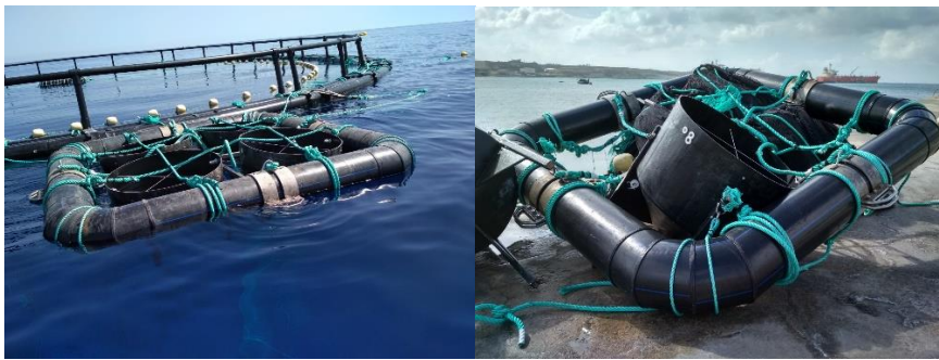
Figure 4. In the top panel a schematic of the in-situ prototype egg incubator made up of 4 Artemia rearing tanks anchored together in a floating frame made of HDPE tubing. The lower left panel shows the incubator placed at sea alongside the broodstock cage. The right panel shows the damaged incubator after a Force 6 storm. A too rigid structure was not applicable to this type of mounting and an alternative protocol was used.
