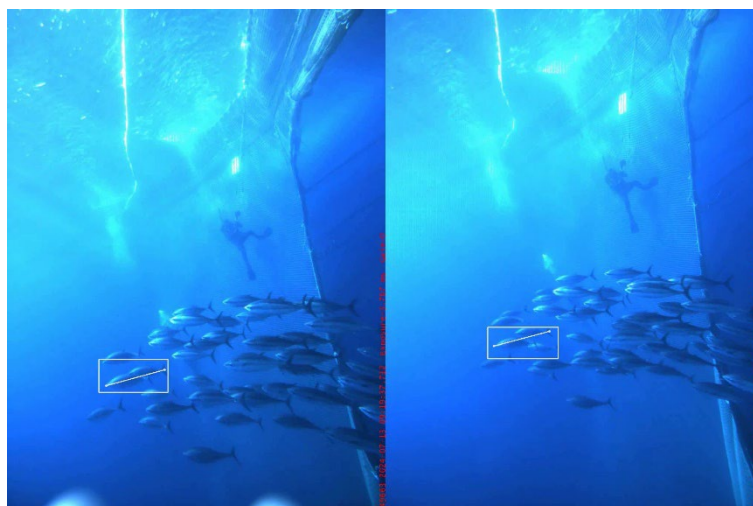
Figure 13. Example of incorrect measurement, where the snout point is placed on one fish and the fork point on a nearby fish.
