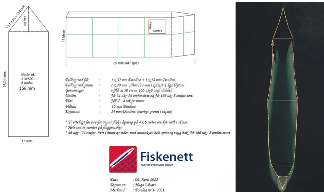
Figure 5: Construction of the transfer cage (left) and aerial view of the transfer cage while towing (right).
