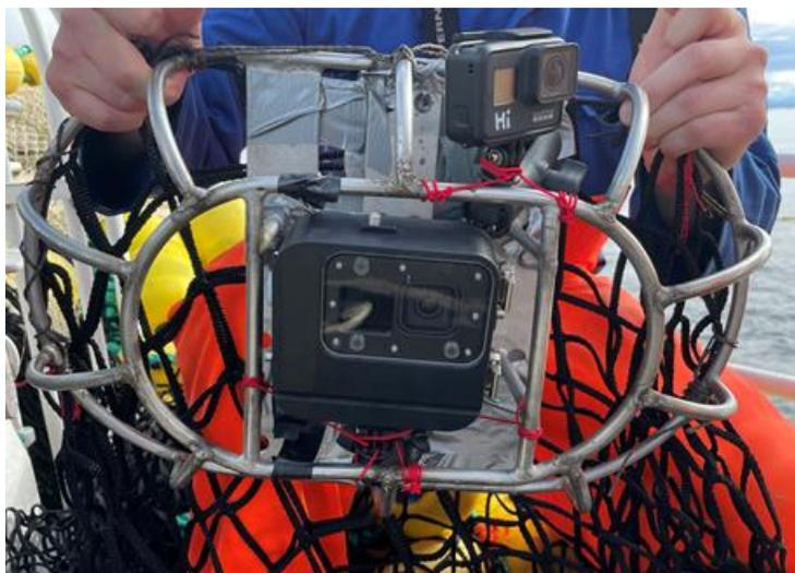
Figure 6: Steel frame with GoPro cameras fixed to the inside of the netting in the channel.
