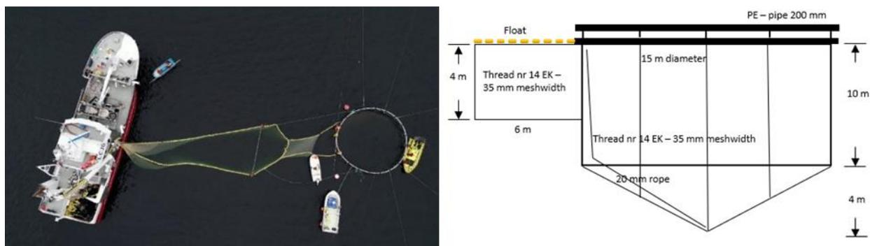
Figure 9: Left: Drone aerial view during the transfer of fish from the transfer cage (centre) to the holding cage (right). Right: Schematics with dimensions of the holding cage.
