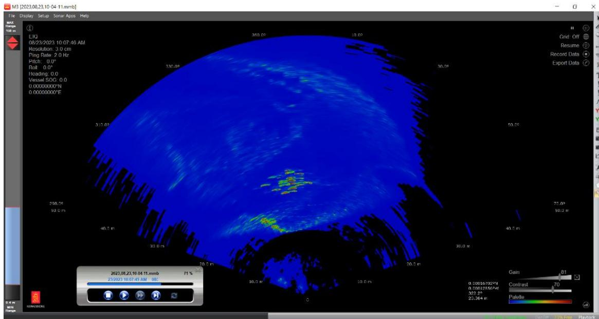
Figure 11: Screen dump from M3 sonar on 23.08.23 during Cast 2. The group of BFT is observed in the center of the image as individually defined oval shaped targets of color between green and orange. Light green and yellow elongated targets correspond to echoes from the purse seine net. Transducer located ca. 15 m from net wall, sampling range of 50 m.
