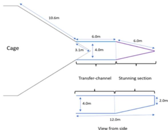
Figure 8: Schematic of the transfer (blue) and stunning channel (purple) attached at the lower end of the transfer cage. Below: side view of the transfer and stunning channel with approximate dimensions.
