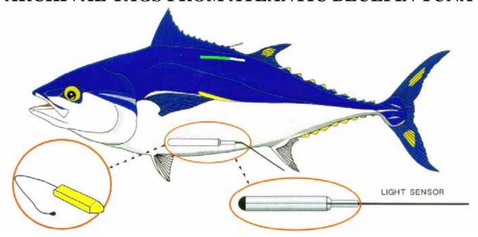
What are archival tags? Archival tags are internal electronic data-recording devices that register information on the daily location of fish through a light sensor. They also provide data on swimming depth, water temperature, and body temperature of the fish. This information is collected on a daily basis and stored in the tag for several years.
