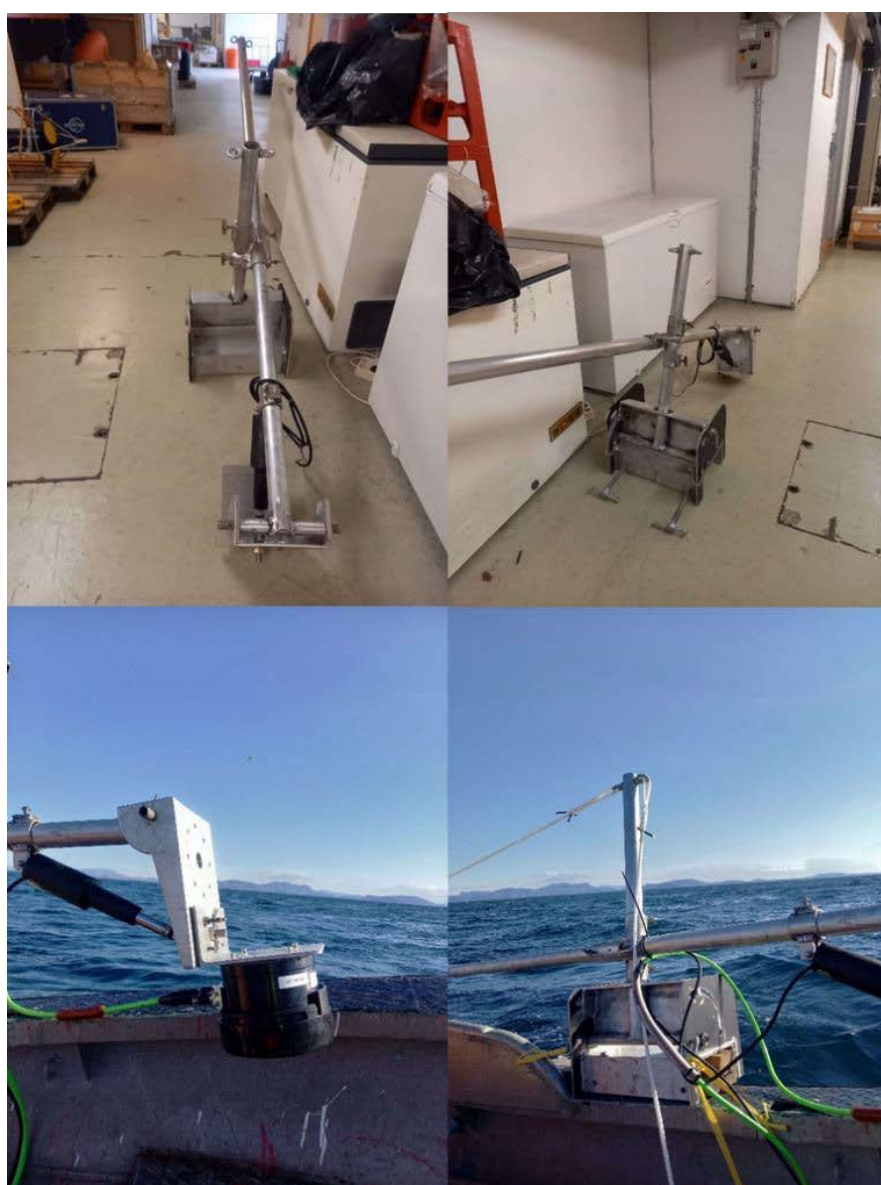
Fig. 2. Pole for mounting M3 sonar. Whole pole with structure to attachment to the skiff and system to allow rest out of water when sailing and deployed when acoustic sampling (top panels). M3 transducer attached to the end of the pole in a platform with an hydraulic arm to allow tilting sonar head (bottom left). Detail of the attachment of the pole system to the skiff side (bottom right).
