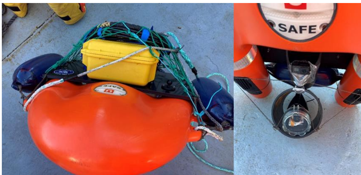
Fig. 6. “USafe” buoy and camera system for monitoring tuna in a purse sein in real-time. Left – the Wireless Mesh Network router inside a water-proof yellow housing, with aerial cable, mounted on type of the “USafe” motorised buoy; Right: the RaspberryPie camera, inside a waterproof housing, mounted beneath the buoy, with a GoPro Hero 7 mounted above. [Image source: Jostein Saltskår].
