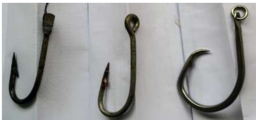
Figure 31. Spatula hooks, an eye on the shank and a hoop on the shank.
