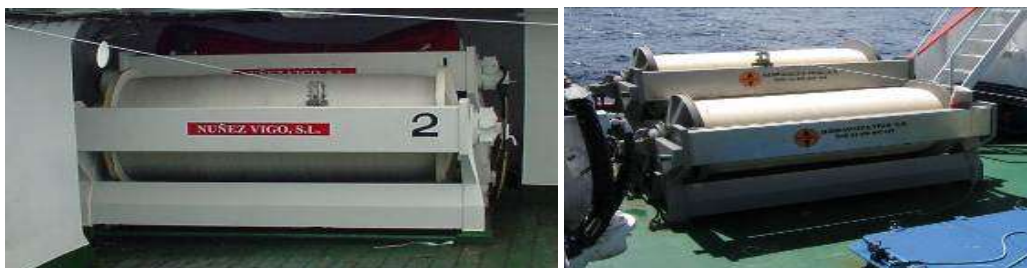
Figure 8. Spool to stow the monofilament main line.
