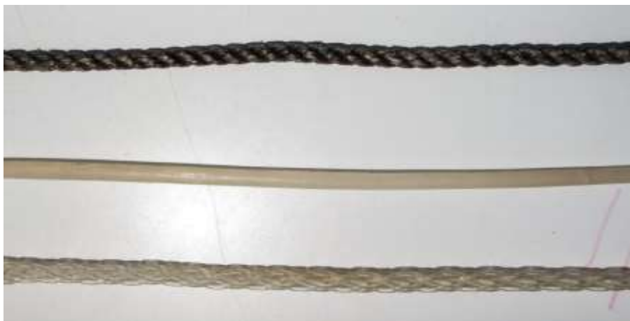
Figure 2. Nylon multifilament main line, polyamide monofilament and woven nylon (from top to bottom).
