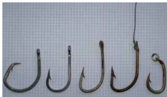
Figure 29. J and circular hooks.
