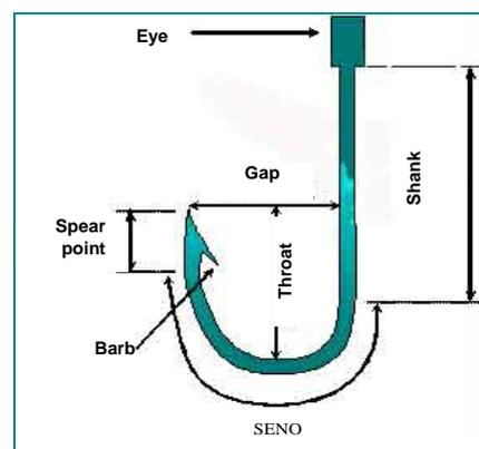
**Figure 1.** Diagram of the parts of a simple hook.
