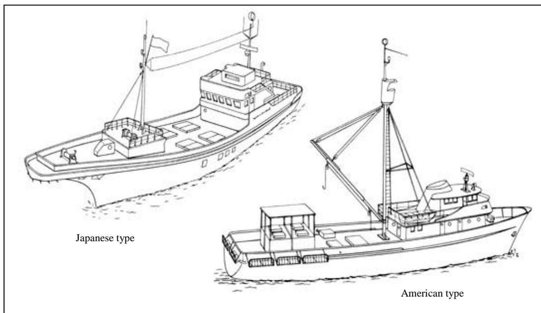
**Figure 2.** Most frequent types of vessel using pole and line (FAO 1986).
