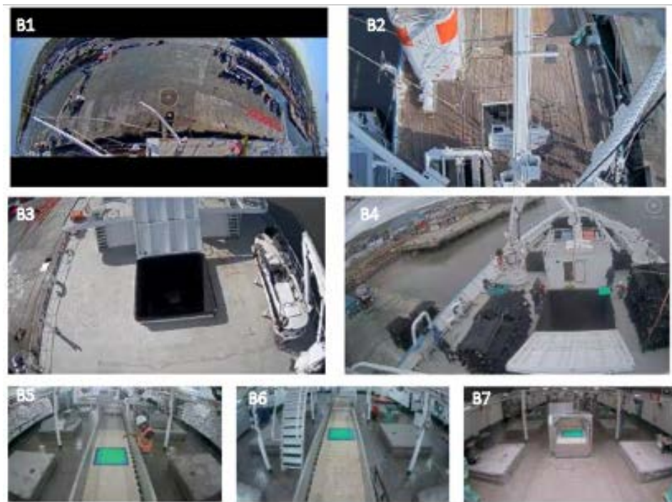
Figure 1. An example of a 7-camera EMS (four in the upper deck and three in the well deck) installed in a purse seiner covering main areas of fishing and fishing handling operations including 1 more camera in the conveyor belt: (B1) 360° Panoramic view camera (e.g port side view), (B2) Crows nest stern view camera, (B3) Working deck crane view camera, (B4) Foredeck view camera, (B5) Conveyor belt stern view camera, (B6) Conveyor belt middle camera, and (B7) Conveyor belt bow camera (source: Digital Observer Services).
