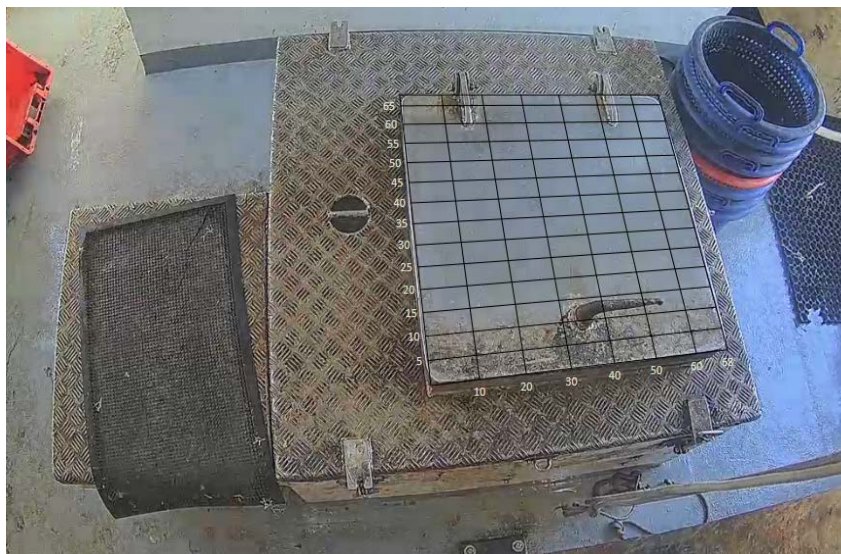
Figure 2. Example of a calibrated hatch onboard a commercial fishing vessel. These areas will vary from vessel to vessel, depending on available surfaces and the species being measured. This image is provided as an example from a non-tuna fishery. For tuna and tuna-like fisheries, the defined areas will have to be larger to accommodate larger species (image source: Centre for Environment Fisheries and Aquaculture Science - Cefas).
