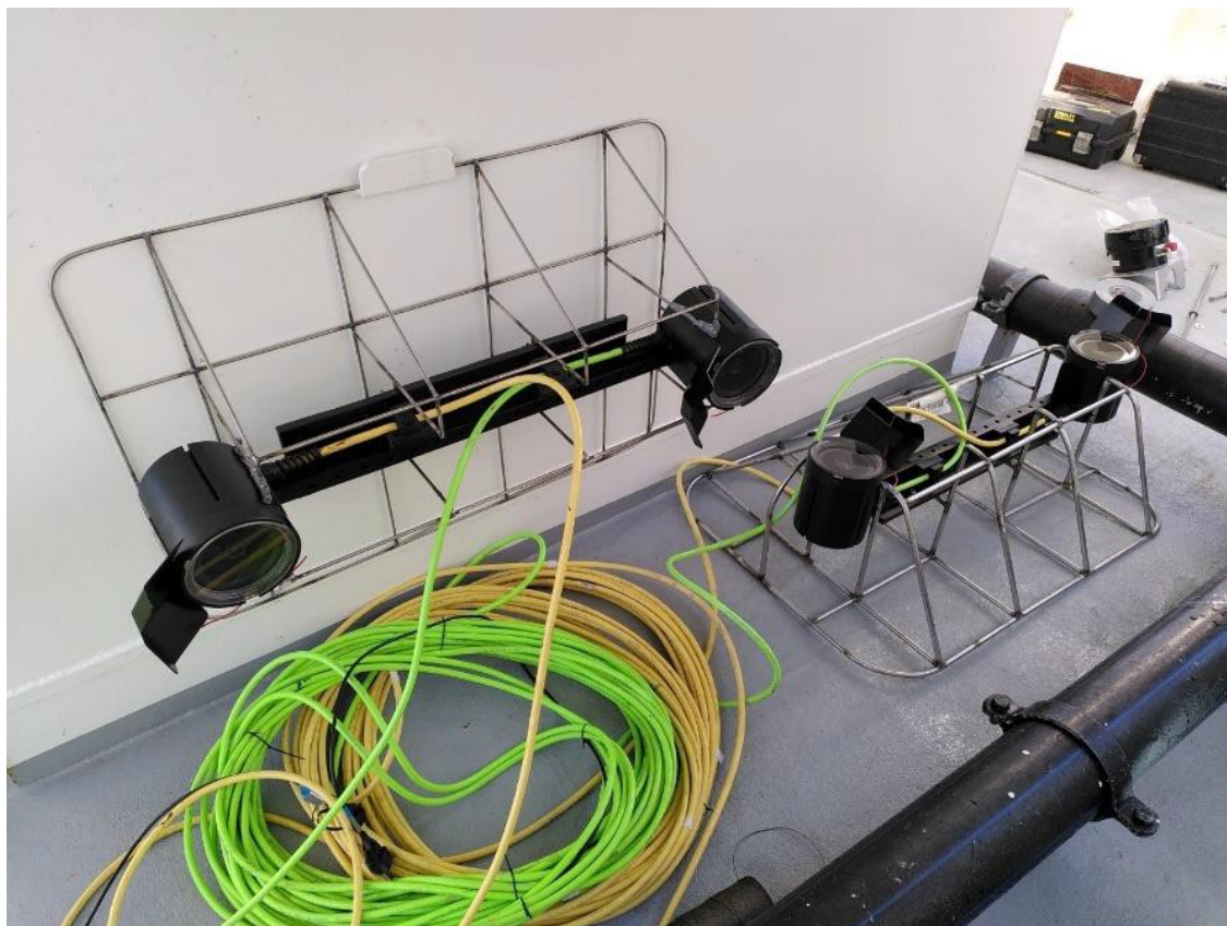
Fig. 5: Stereo camera systems rigged to be set on the side panels of the channel during BFT transfer.
