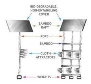
**Figure.** Example of a non-entangling, biodegradable FAD.
