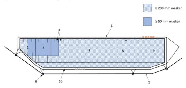
Figure 4: Schematic view of the seine with small mesh panel.
