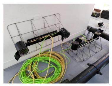
Figure 7: Stereo camera systems rigged prior to deployment on the side panels of the transfer channel.
