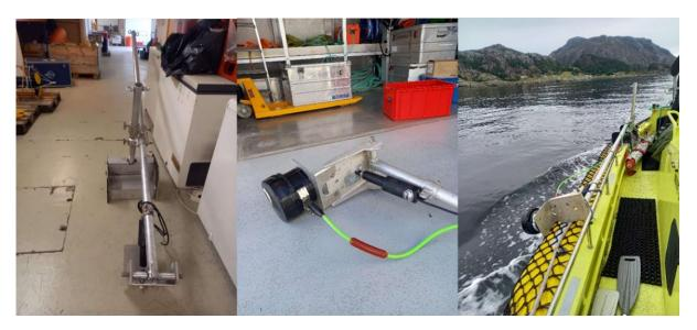
Figure 3: Pole for mounting the M3 sonar. Left: the whole pole with attachment points, including the system to allow retrieval from the water when moving and deployment into the water when acoustic sampling in underway. Middle: M3 transducer mounted to the end of the pole with a hydraulic arm to allow tilting. Right: pole mounted to skiff before deployment.
