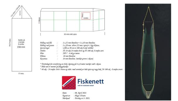
Figure 5: Construction of the transfer cage (left) and aerial view of the transfer cage while towing (right).
