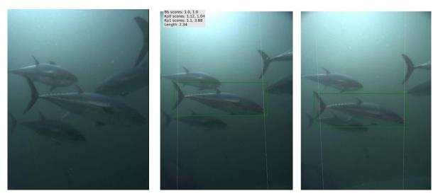
Figure 14: Underwater images obtained using a single camera from the stereo camera system (left) and from using both cameras to estimate length (middle and right).
